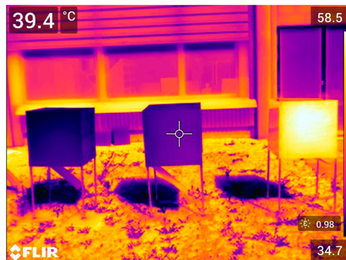
Figure 5. Representative thermographic image measuring external surface temperatures during the experiment.
